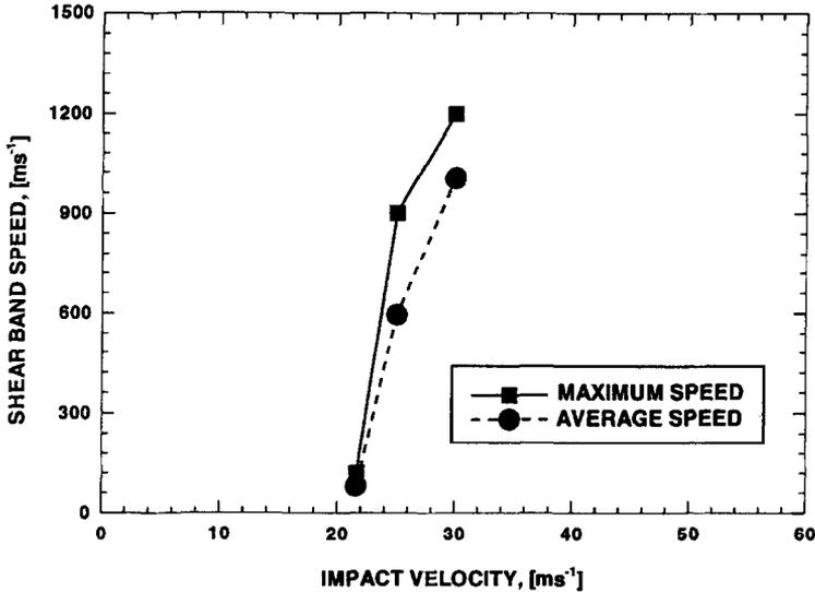
Fig. 20. Maximum and average shear band speeds as functions of impact velocity for C-300 steel.
