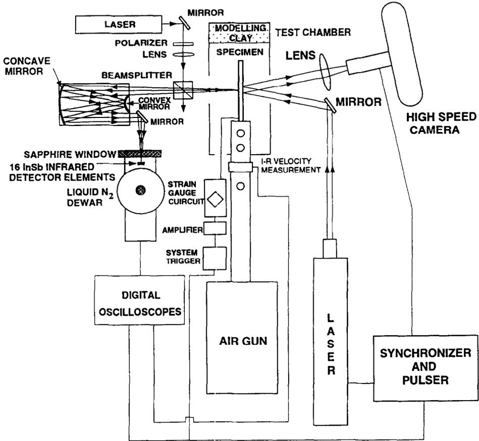
Fig. 6. Experimental apparatus.
