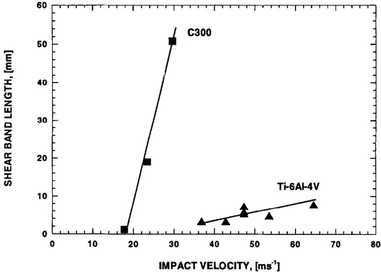
Fig. 15. Maximum shear band length as a function of impact velocity.
