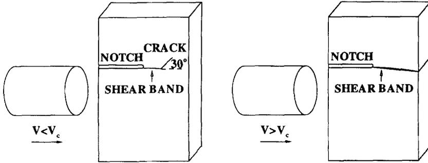
Fig. 1. Asymmetric impact configuration and failure modes.
