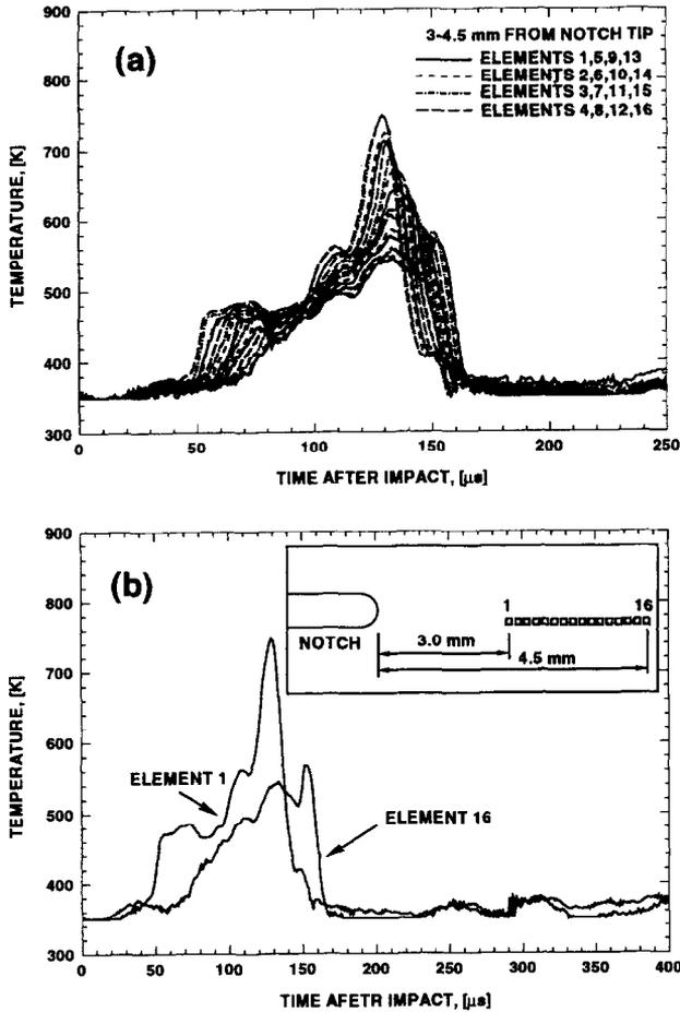
Fig. 14. Temperature profiles at different distances from the notch tip, Ti-6Al-4V,  $V_0 = 64.5 \text{ ms}^{-1}$ .
