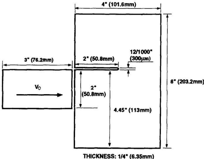
Fig. 2. Dimensions of the specimen used in the asymmetric impact experiment.
