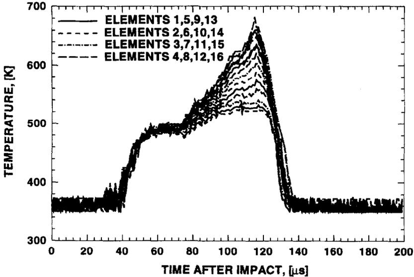
Fig. 10. Temperature profiles around a propagating shear band; Ti-6Al-4V,  $V_0 = 47.3 \text{ ms}^{-1}$ .
