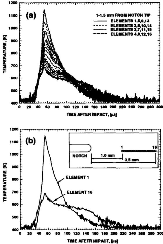
Fig. 13. Temperature profiles at different distances from the notch tip, C-300  $V_0 = 29.7 \text{ ms}^{-1}$ .
