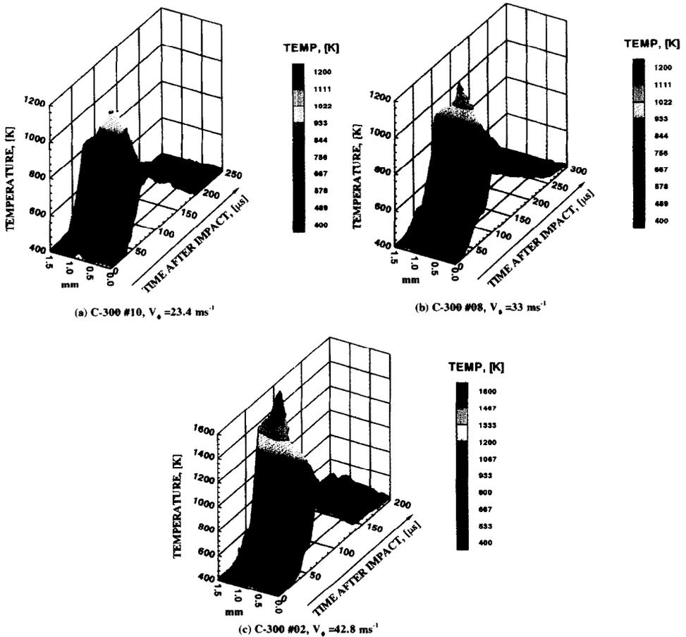
Fig. 9. Temperature profiles around propagating shear bands; C-300 steel. (a) C-300,  $V_0 = 23.4 \text{ ms}^{-1}$ ; (b) C-300,  $V_0 = 33 \text{ ms}^{-1}$ ; (c) C-300,  $V_0 = 42.8 \text{ ms}^{-1}$ .
