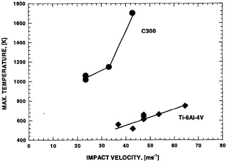
Fig. 12. Maximum temperature as a function of impact velocity.
