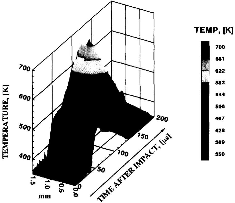
Fig. 11. Temperature profiles around a propagating shear band, Ti-6Al-4V,  $V_0 = 47.3 \text{ ms}^{-1}$ .
