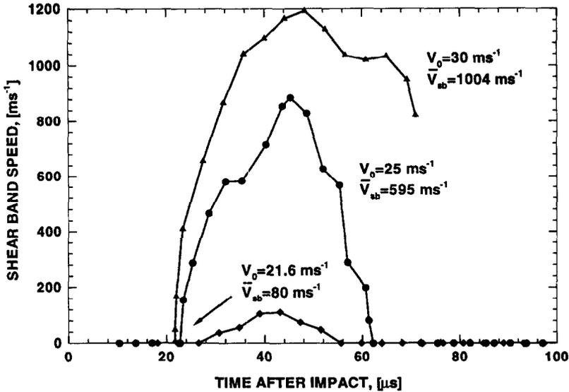
Fig. 19. Shear band speed histories for C-300 at different impact velocities.
