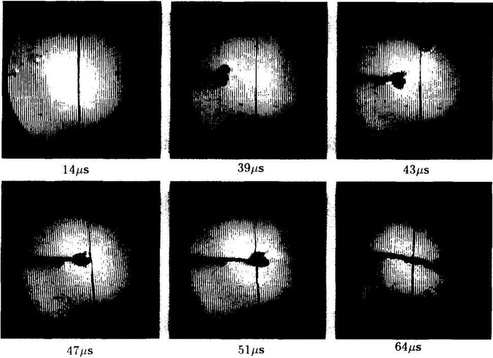
Fig. 17. Images of a propagating shear band recorded by high speed photography for a specimen without a failure mode transition.  $C=300$ ,  $V_0 = 30 \text{ ms}^{-1}$ .
