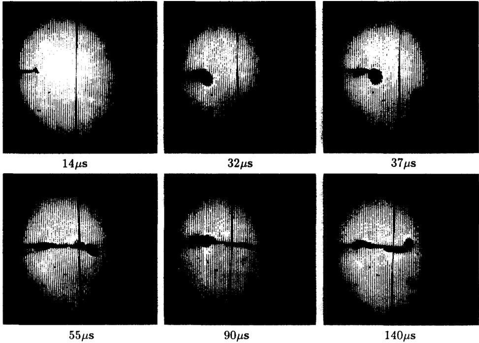
Fig. 16. Images of a propagating shear band and emerging crack recorded by high speed photography, C-300,  $V_0 = 25 \text{ ms}^{-1}$ .
