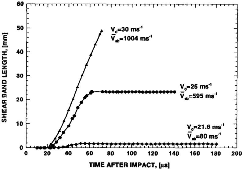
Fig. 18. Shear band length histories for C-300 at different impact velocities.
