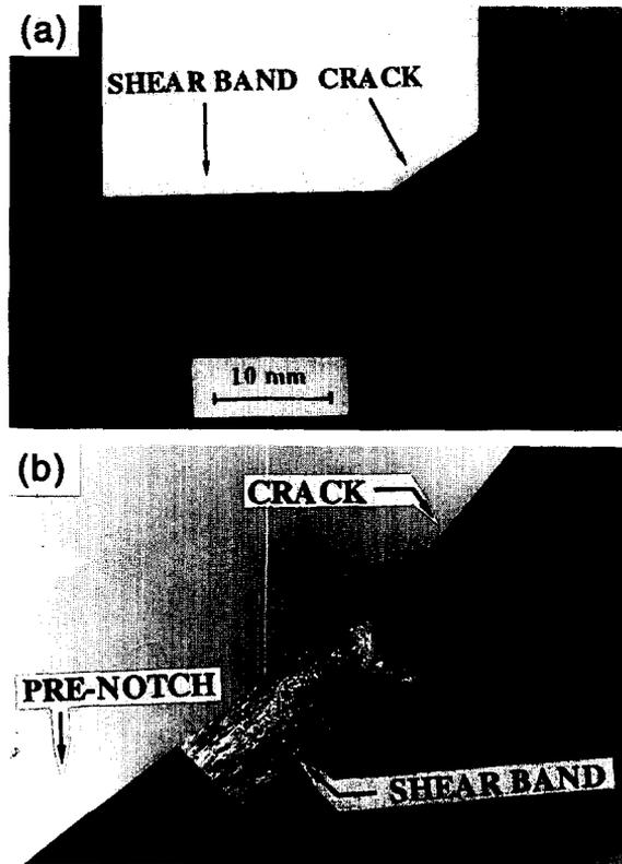
Fig. 3. Failure modes at intermediate impact velocities,  $V_0 = 23.4 \text{ ms}^{-1}$ , C-300 steel.
