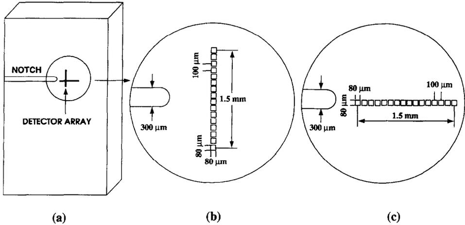
Fig. 7. A schematic illustration of the infrared temperature measurement schemes used in the experiments.
